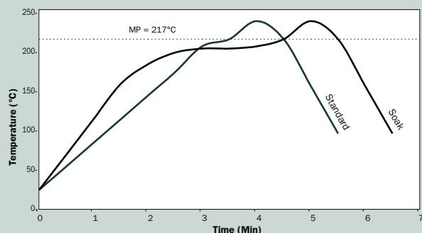
The stated profile recommendations apply to most Pb-Free alloys in the Sn/Ag/Cu (SAC) alloy system, including SAC 305 (96.5Sn/3.0Ag/0.5Cu). This can be used as a general guideline in establishing a reflow profile when using **Indium5.8LS** Solder Paste. Deviations from these recommendations are acceptable, and may be necessary, based on specific process requirements, including board size, thickness & density.
