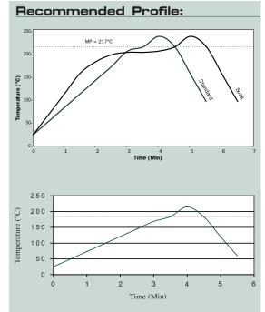
Peak reflow temperature should be <250°C in an air or nitrogen atmosphere, with a linear ramp up to approximately 30°C above the solidus temperature.
