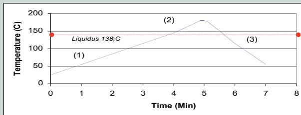
This profile is designed for use with Indalloy #281 and can serve as a general guideline in establishing a reflow profile for use with other alloys. Adjustments to this profile may be necessary based on specific process requirements.
